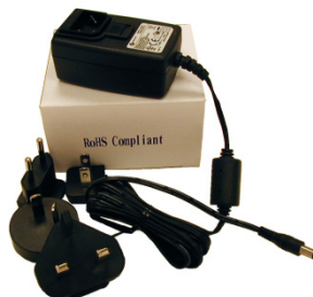
Figure 4. AC power adapter with interchangeable AC plugs
